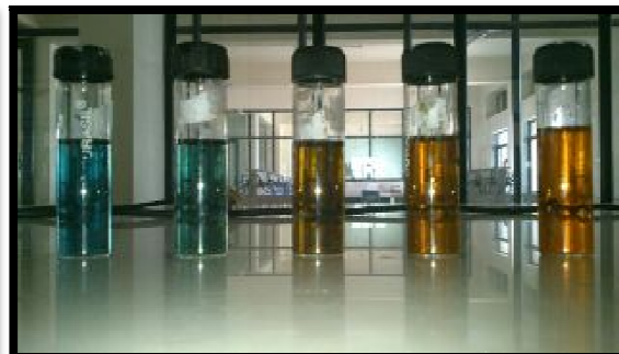
Image 2b: shows color formation in dichromate method of date sample
