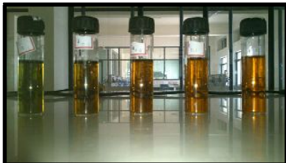
Image 2a: shows color formation in dichromate method of fig sample
